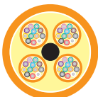
48-fibers (4 tubes of 12-fibers)
