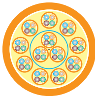
48-fibers (12 tubes of 4-fibers)
