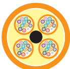
48-fibers (4 tubes of 12-fibers)
