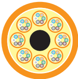
48-fibers (8 tubes of 6-fibers)
