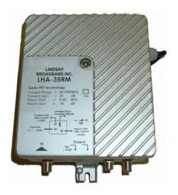
LHA series CATV Distribution Amplifiers with active return are broadband indoor GaAs-Fet / PushPull distribution amplifiers designed for RF distribution systems such as those in Cable Television Apartments, Hotels, Hospitals and other applications where a high quality low noise figure amplifier is necessary to amplify the signals in both the forward and return paths.
