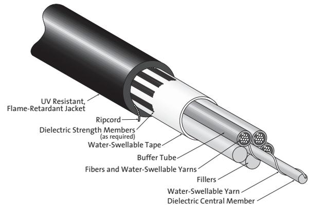
FREEDM Loose Tube Gel-Free Cable | Drawing ZA-1894
