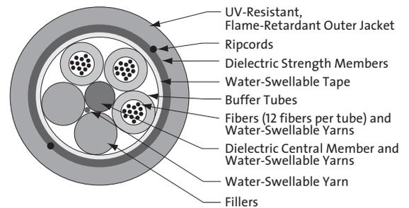
36-Fiber FREEDM Loose Tube Gel-Free Cable | Drawing ZA-1596
