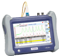
Handheld instrument for testing 10 G Ethernet and fiber networks
