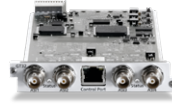
GT32 ASI to IP/IP to ASI 4x ASI input or output, demux & passthrough
