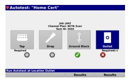
Multi-user support allows technicians that work in various territories to easily switch channel plans and standardized autotest apps and test limits or login as a completely different user. Connecting to ViewPoint allows techs to upload job data in near real-time as well as transmit and receive channel plans, autotests, and firmware.
