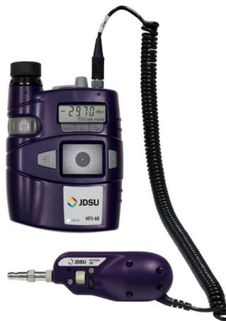
The HP3-60-P4 system, derived from the popular HD3 series, provides high-quality image resolution in a compact, portable design. The integrated power meter offers quick, easy, and convenient field measurement of optical power and attenuation. Easy push-button operation makes the device simple and straightforward, while the inspect-test process establishes optimal workflow practices.
