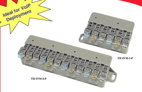
The TII Switchable Voice Module (SVM) contains a microprocessor controlled circuit that provides seamless switching from Telco service to digital phone service. The second ringing voltage appearance on the digital phone service initiates the switch over. The TII SVM utilizes gel-sealed insulation displacement terminations that provide reliable all weather connectivity.
